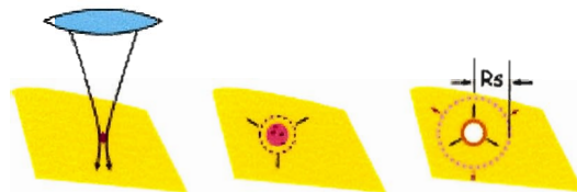
Figure 8: Laser-induced optical breakdown occurs at the beam focus. A high-density plasma then expands outward where R_s is the radius at which the shock wave has relaxed to an ordinary acoustic wave.
