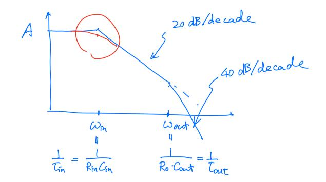
Using the concept of impedance, it's easy to derive the transfer function
