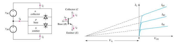
The schematic structure, symbol, and the current-voltage (I-V) characteristics of a BJT are shown above. The collector current,  $I_C$ , is controlled by base current,  $I_B$ . The flat part of the I-V curves is call "forward active" region. The flatness of the  $I_C$  curves is described by "Early voltage",  $V_A$ :
