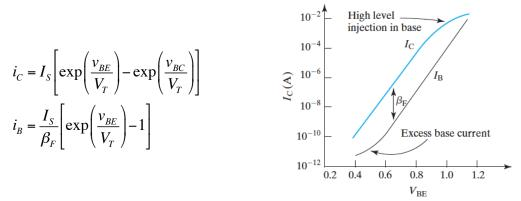
In semi-log plot of  $I_B$  and  $I_C$  vs.  $V_{BE}$ , both are linear curves except for very low and very high currents. The ratio between them is the current gain,  $\beta$ . **MOSFET (Metal-oxide-semiconductor field effect transistors):**
