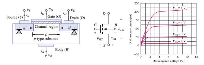
The schematic structure, symbol, and current-voltage (I-V) characteristics of an N-channel MOSFET (NMOS) are shown above. The current flowing from drain to source,  $I_{DS}$ , (or electrons moving from source to drain) is controlled by the gate-source voltage,  $V_{GS}$ . On the "flat" part of the I-V curves, the so-called "saturation region", is described by the following equation:
