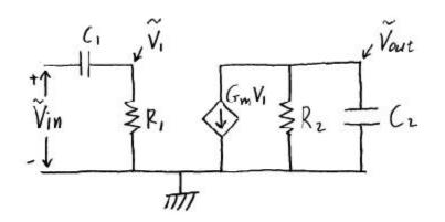
b) Plot amplitude and phase Bode plots when  $R_1=10k\Omega$ ,  $C_1=0.01\mu$ F,  $R_2=1k\Omega$ ,  $C_2=0.001\mu$ F,  $G_m=0.01S$ . (10 pts for each plot).
