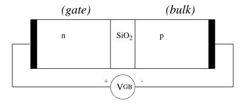
a. Calculate the depth of the depletion regions when  $V_{GB} = 0$ . (10pts)
