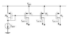
By mixing n-channel and p-channel diode-connected devices, we can produce current sinks and sources from a reference current connected to V<sub>DD</sub> or ground.
