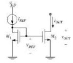
• Intuitively,  $V_{REF}$  is set by  $I_{REF}$  and determines the output current of  $M_2$
