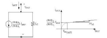
The model is only valid for  $v_{DS} = v_{OUT} > v_{DS(SAT)} = V_{GS} - V_{Tn}$
