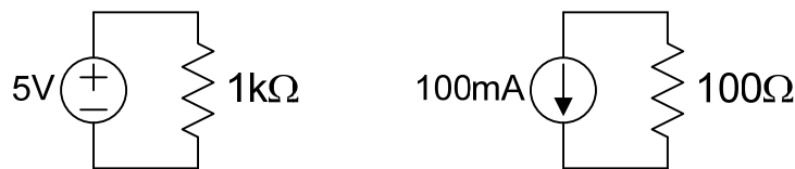
Figure 1 Circuit symbols and diagrams for a 5V voltage and a 100mA current supply. In this example, both sources are loaded by resistors, but would power a more complicated load in a practical application.
