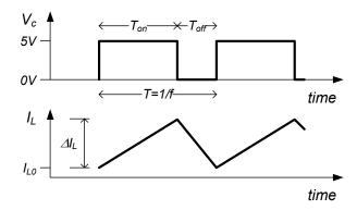
Since voltage is proportional to the slope of the current, we note intuitively that reducing the ratio of  $T_{off}/T_{on}$  results in higher output voltage  $V_{out}$ . This is because the positive slope is proportional to  $V_{in}$  and the negative slope of the decreasing current is proportional to  $V_{out}$  -  $V_{in}$ . In the laboratory we will analyze this relationship quantitatively.
