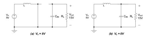
In situation (a),  $V_c$ =5V, the supply voltage  $V_{in}$  appears across the inductor. From the differential equation for inductance we observe that inductors integrate voltage. Therefore the inductor current  $I_L$  is a ramp with slope determined by  $V_{in}$  and L. In situation (b) the inductor again integrates the voltage
