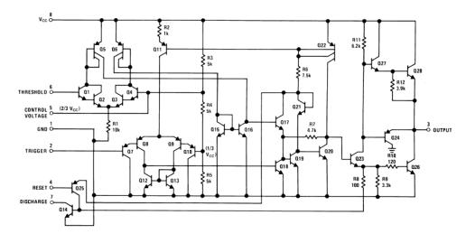
Since you have not studied capacitors and inductors in lecture (yet), you will be responsible for just building two simple circuits in this lab. The first circuit is the above mentioned 555 timer circuit. The fact that you simply apply power to the chip to get a square wave output should be fascinating:
