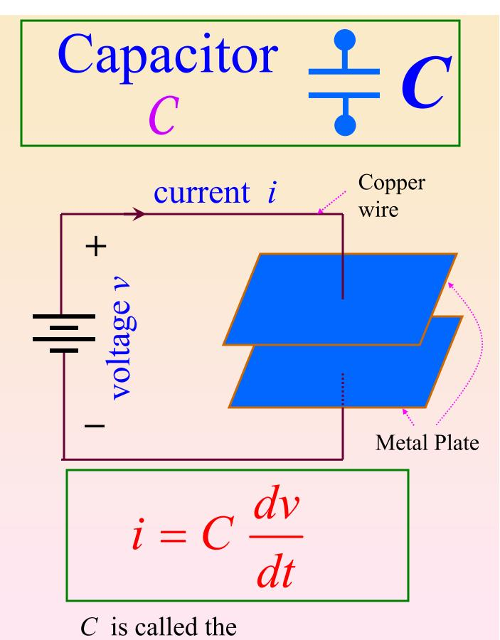
Capacitance of the Capacitor C
