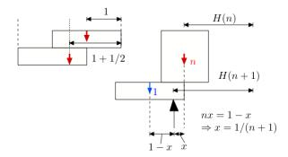
The cards have width 2. Induction shows that the center of gravity after *n* cards is H(n) away from the right-most edge.
