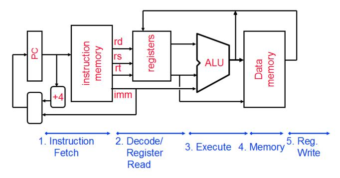
rd, rs, and rt are 5 bit wires, imm is a 16 bit wire. All other wires are 32 bits wide.
