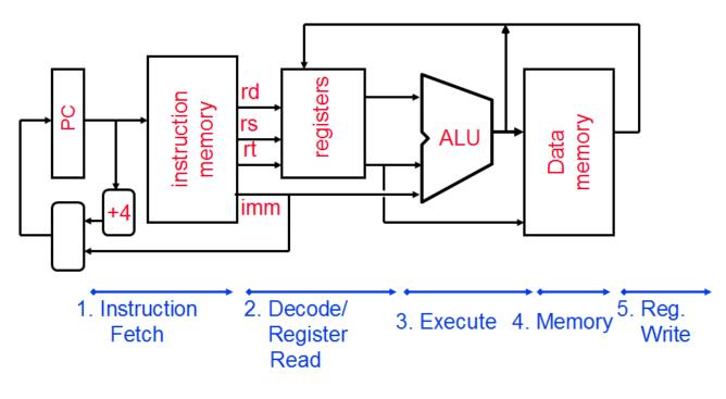
rd, rs, and rt are 5 bit wires, imm is a 16 bit wire. All other wires are 32 bits wide.
