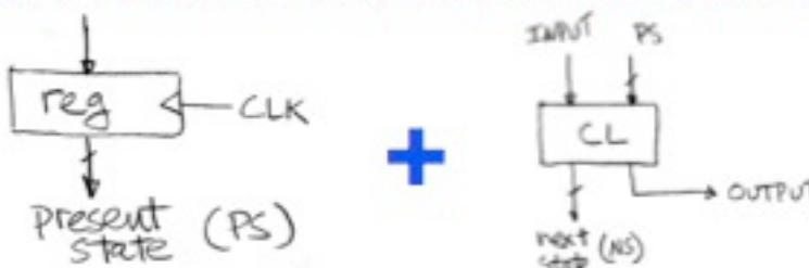
Combinational logic circuit is used to implement a function maps from *present state* and *input* to *next state* and *output*.
