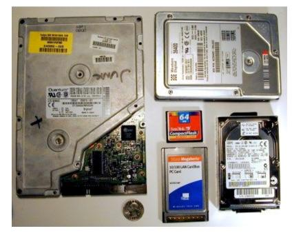
The five most popular internal form factors for PC hard disks. Clockwise from the left: 5.25", 3.5", 2.5", PC Card and CompactFlash.
