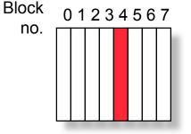
Direct mapped: block 12 can go only into block 4 (12 mod 8) Block 0 1 2 3 4 5 6 7 no. Set Set Set Set 0 1 2 3 Set associative: block 12 can go anywhere in set 0 (12 mod 4)
