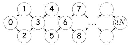
Treat 0 as the root and do recursive traversal down the two edges out of each node:  $\Theta(2^N)$  operations!
