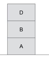
Stack Machine - a processor or virtual machine that computes by modifying values in a stack. Has very simple instructions!
