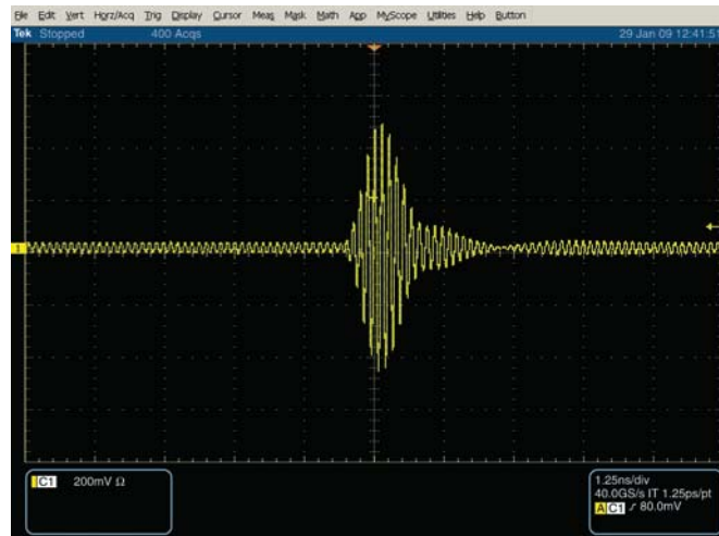
Figure 3 – A UWB pulse consists of a 7.68-GHz carrier wave with a Gaussian envelope.
