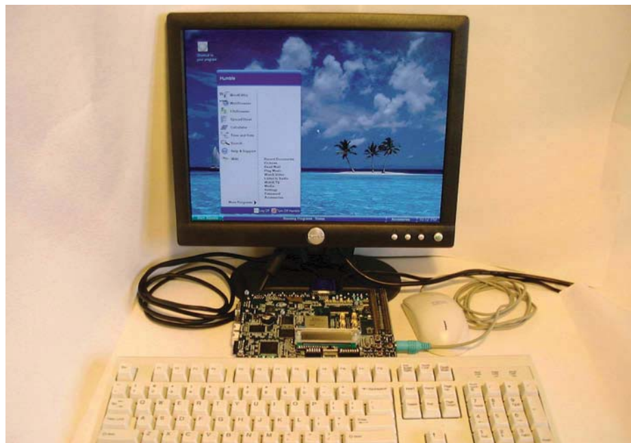
Figure 1 – The HUMBLE PC turns on in a second, thanks to a microprocessor-less architecture that has no need to fetch instructions.
