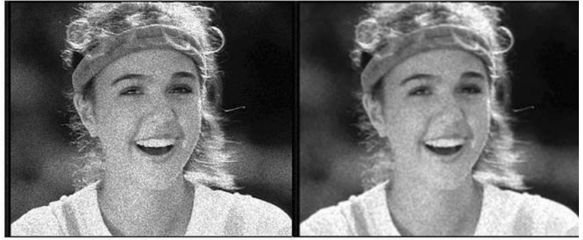
Figure 6 – Speckle noise affects the image on the left; on the right side is the filtered image.
