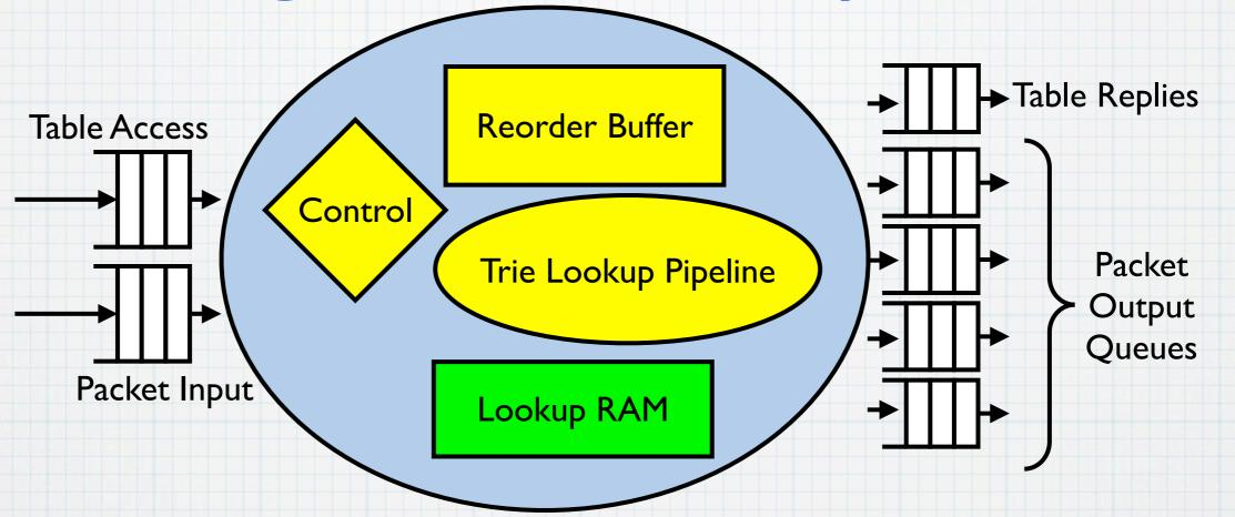
The reorder buffer, the trie lookup pipeline's registers, and any control state are microarchitectural state that should not affect function as viewed from outside
