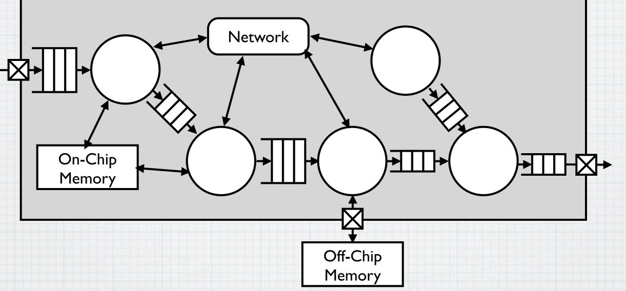
System performance limited by application requirements, on-chip performance, off-chip I/O, or power/energy
