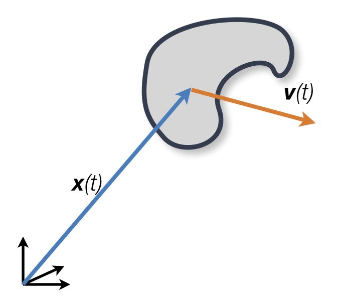
Center of mass behaves like a mass point with total mass of the body  $M = \sum m_i$  $\mathbf{x}_{cm} = \frac{\sum_{i} m_i \mathbf{x}_i}{M}$  $=\frac{\sum_{i}m_{i}\mathbf{v_{i}}}{M}$  $\mathbf{v}_{cm}$  =  $\mathbf{a}_{cm} = \frac{\sum_{i} m_i \mathbf{a_i}}{M}$
