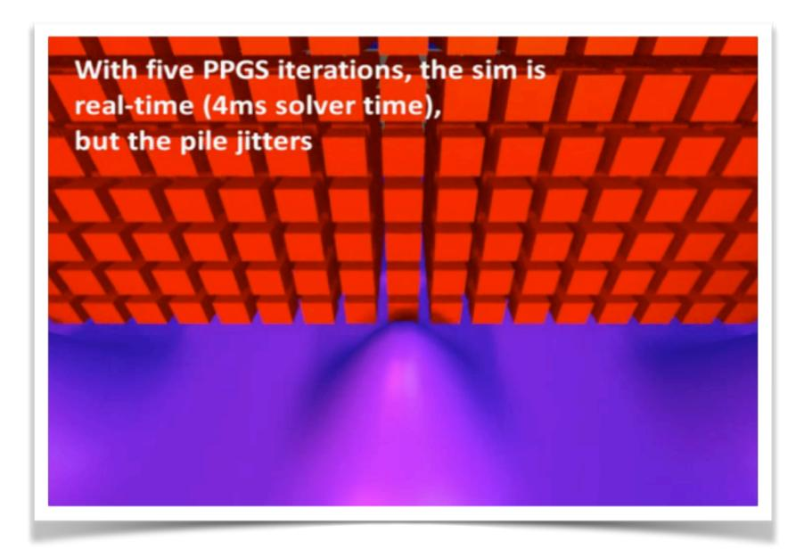
Tonge et al. 2012 Mass splitting for jitterfree RB simulations
