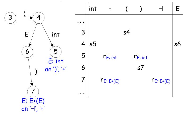
Legend: 's N' means "shift (or go to) state N."  $r_P$  means "reduce using production P." blank entries indicate errors.
