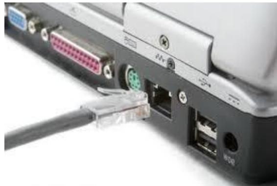
Ethernet cable and port
