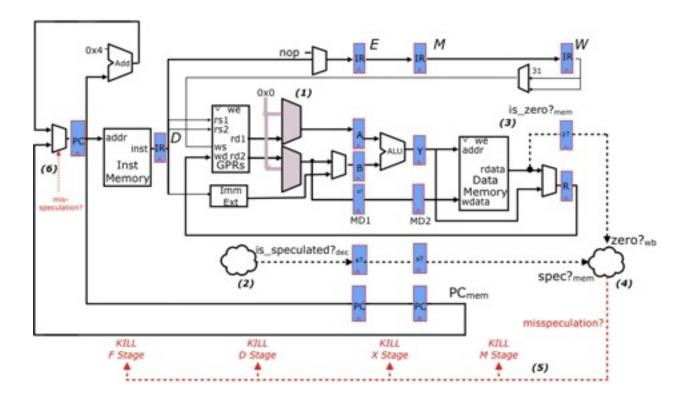
*Note*: for the sake of clarity, some of the bypass lines and control signals have been removed *from the drawing*, but this is still a fully bypassed pipeline.
