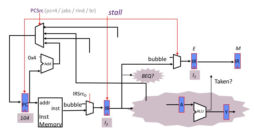
096ADDBranch condition is not known until the100BEQ x1,x2 +200execute stage104ADDwhat action should be taken in the300ADDdecode stage ?
