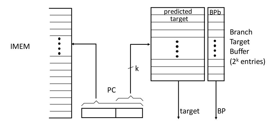
BP bits are stored with the predicted target address.
