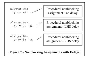
Adding delays to the left-hand-side (LHS) of nonblocking assignments (as shown in Figure 7) to model combinational logic is flawed.
