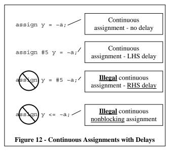
Adding delays to continuous assignments (as shown in Figure 12) accurately models combinational logic with *inertial delays* and is a recommended coding style.
