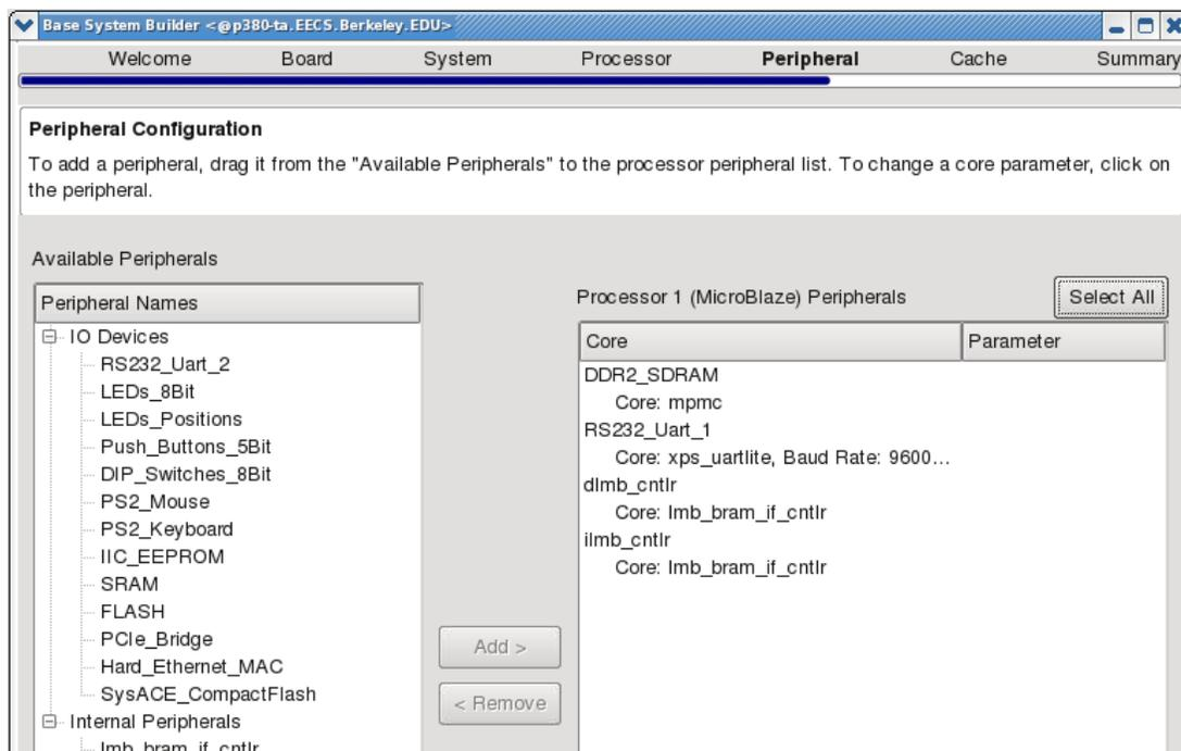
Similar to Lab5B, the RS232\_Uart\_1 will be used to communicate with the host workstation, while the `lmb_cntlr` and `ilmb_cntlr` are used by the processor to access the local memory (Block RAM). The DRAM controller added has multiple ports. We can thus have a coprocessor writing into one port, while the MicroBlaze and other coprocessors reading from other ports.
