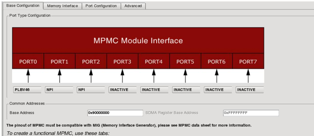
Select `Hardware` → `Configure Coprocessor` to add the newly created coprocessors to the system (readcop first, then writecop). They are now connected to the MicroBlaze through FSL interface, but the connections to the NPI interfaces in MPMC have yet to be established.
