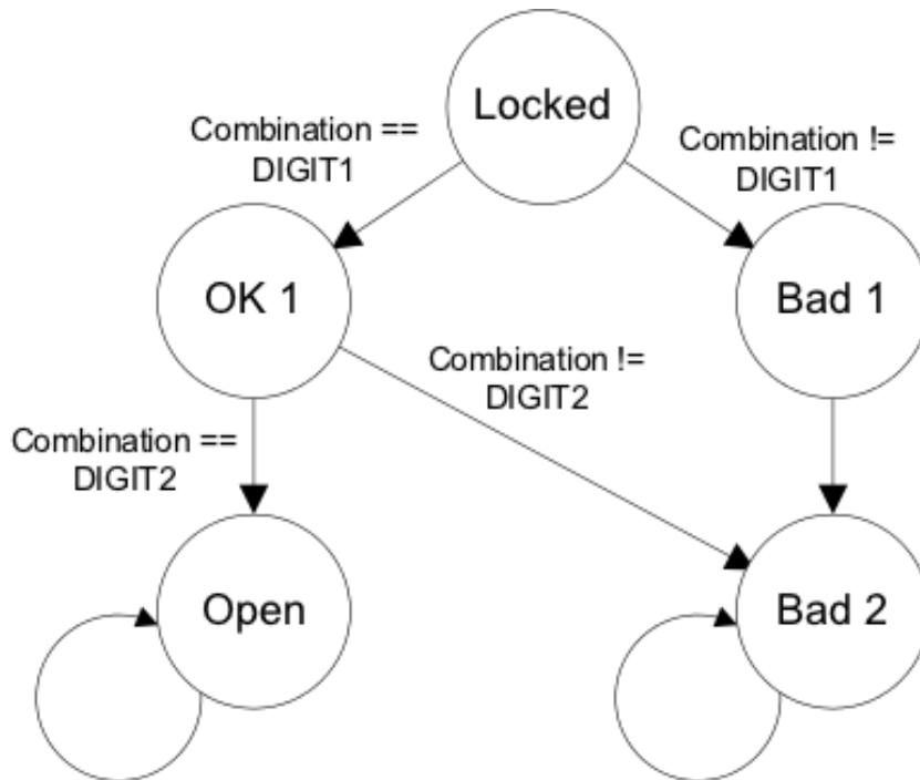
Figure 2 Lab2Lock FSM
