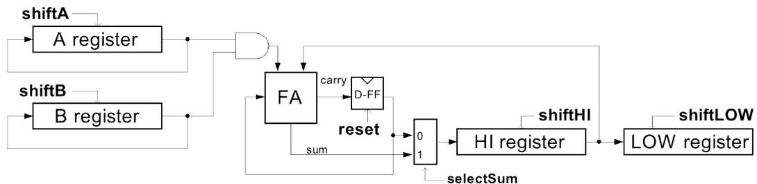
To better understand this circuit, trace (write down the contents of registers at every cycle) the multiplication of 4'd5 by 4'b9 through a 4-bit bit-serial multiplier.
