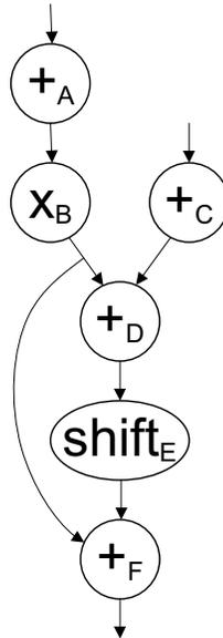
Use modulo scheduling to show how to complete four iterations of the loop in the minimum number of cycles. Show your work. Then, fill in the chart shown below the unique integer node numbers from the graph. Use subscripts (1, 2, 3, and 4) to indicate the iteration number. For instance, "C<sub>2</sub>" indicates node C of iteration 2.
