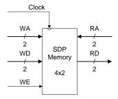
2. Implement a 8x2 **three-port** memory with 2 asynchronous read ports, and 1 write port. Use the space below.
