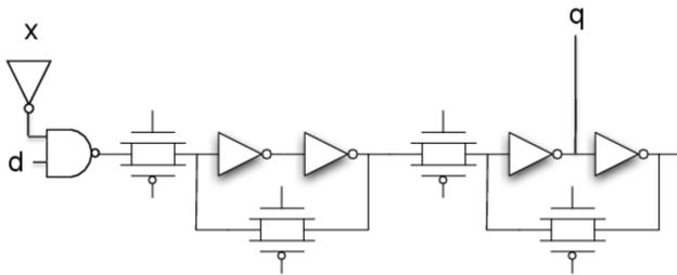
c. Modify the D-master-slave FF circuit below, using minimum number of gates, to add a clock enable.
