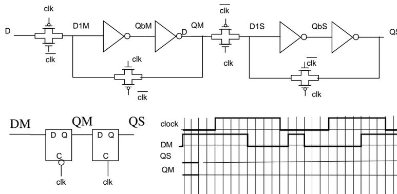
a. Draw a timing diagram for the D master-slave FF circuit below, assuming unit delay through the inverters and transmission gates, and showing signals  $clk$ ,  $DM$ ,  $D1M$ ,  $QbM$ ,  $QM$ ,  $D1S$ ,  $QbS$ ,  $QS$ .
