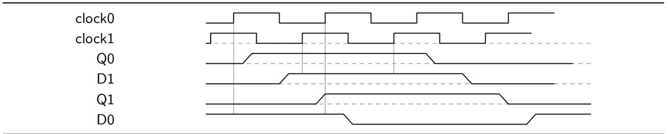
From the timing diagram we need to check setup and hold times for both flip flops.
