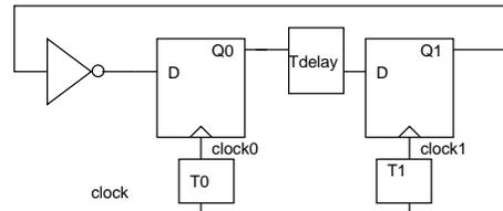
a. With delay  $T_0 = T_1 = 0$  ns, what is the maximum clock speed?
