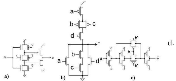
Implement the function  $y = \overline{(a + b)(c + d)}$  using CMOS transistors with the minimum number of transistors.
