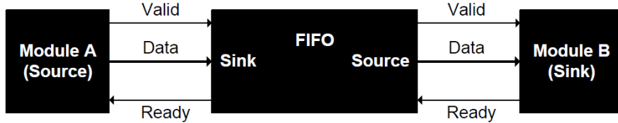
Figure 8 A FIFO functioning as both a source and sink
