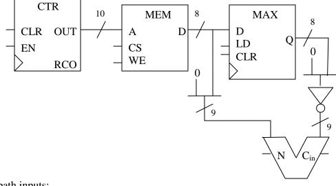
b) Datapath inputs: CTR\_CLR, CTR\_EN MEM\_CS, MEM\_WE MAX\_LD, MAX\_CLR ALU\_Cin Datapath outputs: CTR\_RCO, ALU\_N
