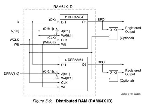
If two dual-port 64 x 1-bit modules are built, the two RAM64X1D primitives can occupy a SLICEM, as long as they share the same clock, write enable, and shared read and write port address inputs. This configuration equates to 64 x 2-bit dual-port distributed RAM.
