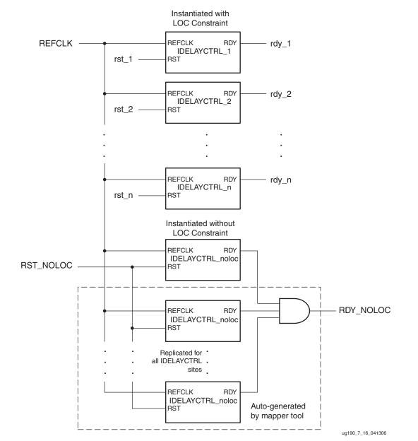
*Figure 7-21:* **Mixed Instantiation of IDELAYCTRL Elements**
