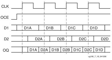
Figure 7-23: Output DDR Timing in OPPOSITE\_EDGE Mode
