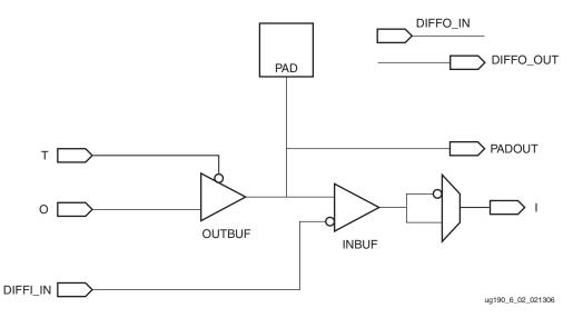
Figure 6-2: Basic IOB Diagram
