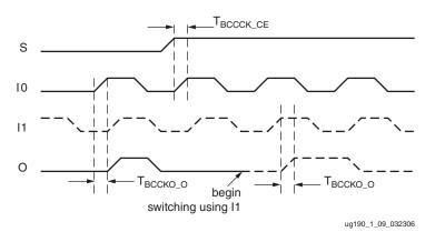
Figure 1-9: BUFGMUX Timing Diagram
