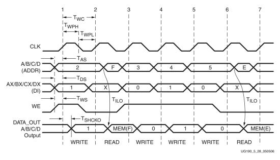
Figure 5-28: Slice Distributed RAM Timing Characteristics
