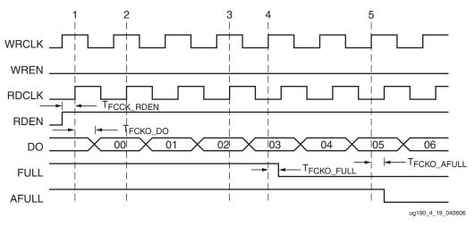
Figure 4-23: Reading From a Full FIFO
