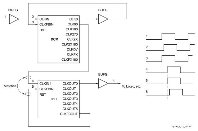
Figure 3-13: DCM Driving a PLL
