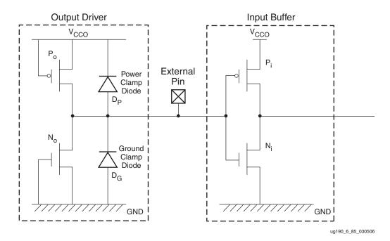
Figure 6-91: Virtex-5 FPGA I/O: 3-State Output Driver
