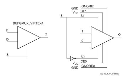
Figure 1-11: BUFGMUX\_VIRTEX4 as BUFGCTRL
