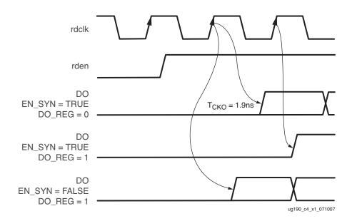
Figure 4-16: Synchronous FIFO Data Timing Diagram
