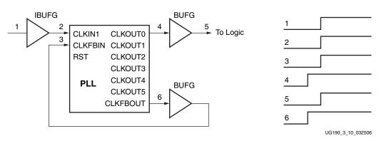
Figure 3-10: Clock Deskew Using Two BUFGs
