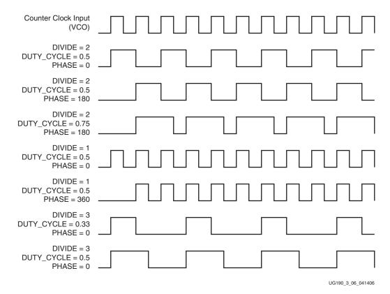
Figure 3-6: Output Counter Clock Synthesis Examples
