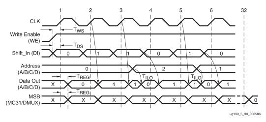
Figure 5-30: Slice SRL Timing Characteristics
