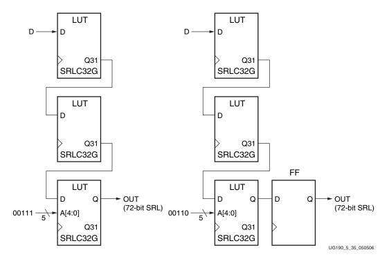
Figure 5-35: Example Static-Length Shift Register
