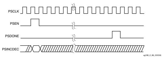
Figure 2-6: Phase-Shift Timing Diagram
