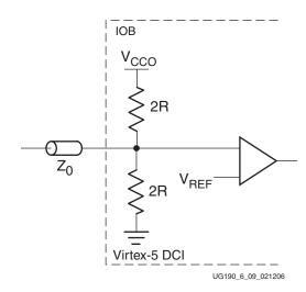
Figure 6-11 illustrates split termination inside a Virtex-5 device.
