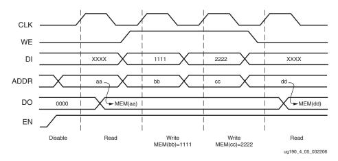
Figure 4-4: NO\_CHANGE Mode Waveforms
