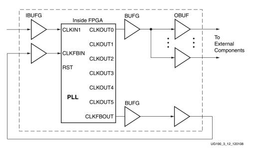
Figure 3-12: Zero Delay Buffer
