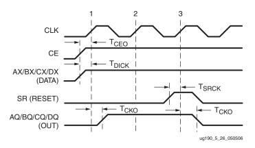
Figure 5-26: General Slice Timing Characteristics
