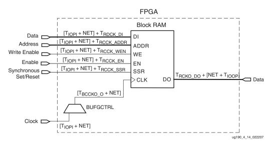
Figure 4-15: Block RAM Timing Model
