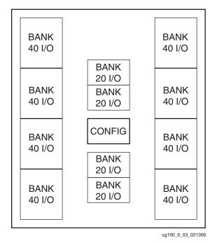
Figure 6-3: Virtex-5 FPGA XC5VLX30 I/O Banks
