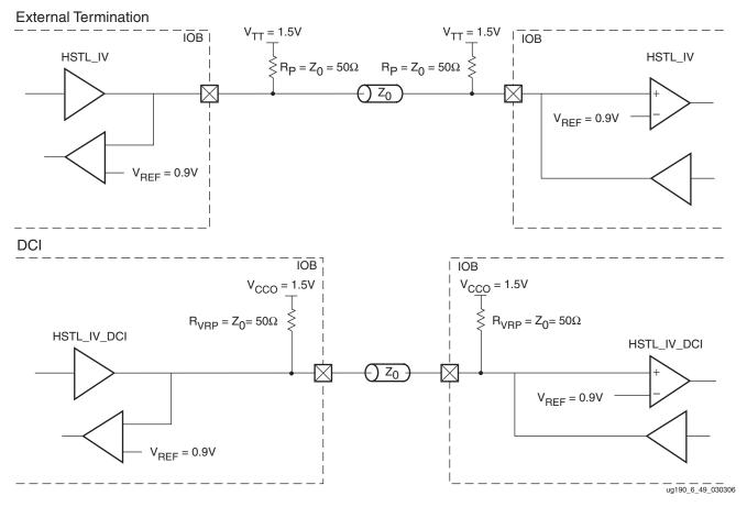
Figure 6-51: HSTL Class IV Bidirectional Termination
