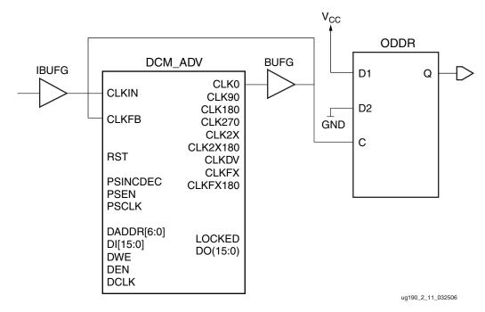
Figure 2-10: Board-Level Clock with Internal Feedback
