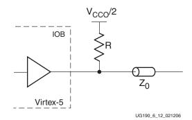
Figure 6-14: Driver with Termination to V<sub>CCO</sub>/2 without DCI
