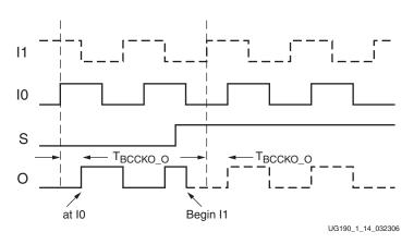
Figure 1-14: Asynchronous Mux Timing Diagram
