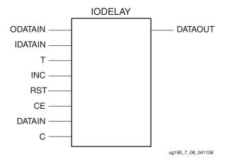
Figure 7-8: IODELAY Primitive
