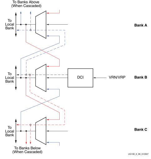
Figure 6-5 shows DCI cascading support over multiple banks. Bank B is the master bank.
