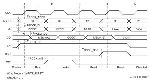
Figure 4-14: Block RAM Timing Diagram
