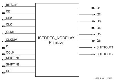
Figure 8-2: ISERDES\_NODELAY Primitive
