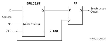
Figure 5-34: Synchronous Shift Register
