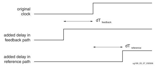
Figure 3-7: Basic Output Clock Shifting
