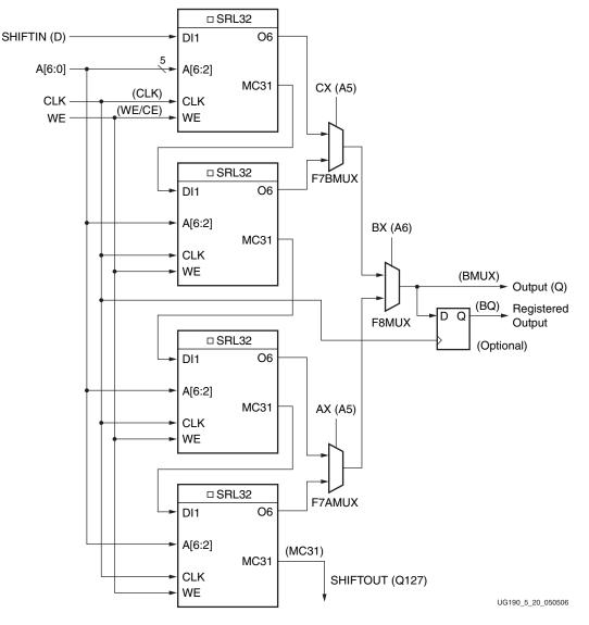
Figure 5-20: 128-bit Shift Register Configuration
