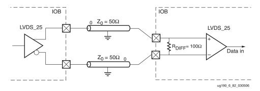
Figure 6-88: LVDS\_25 With DIFF\_TERM Receiver Termination
