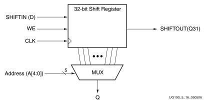
Figure 5-16: Representation of a Shift Register
