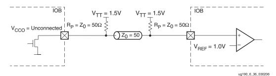
Figure 6-38: GTL+ with External Parallel Termination and Unconnected V<sub>CCO</sub>
