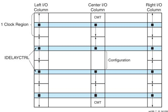
Figure 7-17: Relative Locations of IDELAYCTRL Modules
