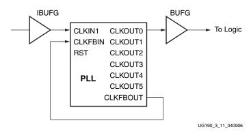
Figure 3-11: PLL with Internal Feedback
