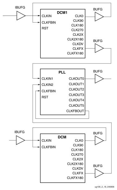
*Figure 2-16:* **Two DCMs Driving a PLL**
