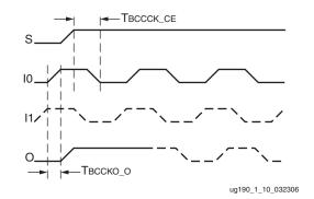
Figure 1-10: BUFGMUX\_1 Timing Diagram
