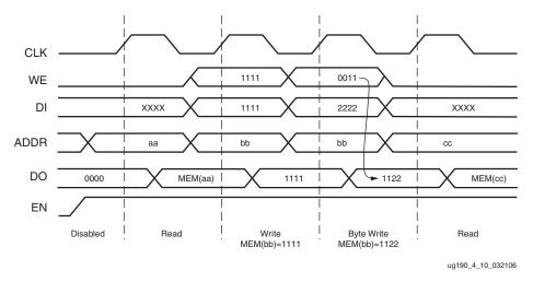
Figure 4-8: Byte-wide Write Operation Waveforms (x36 WRITE\_FIRST)
