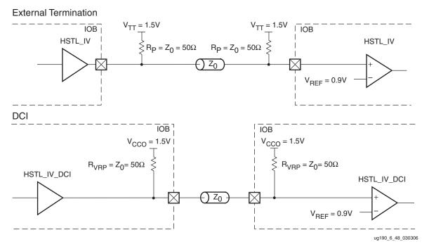
Figure 6-50: HSTL Class IV Unidirectional Termination
