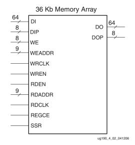
Figure 4-6: Simple Dual-Port Data Flow
