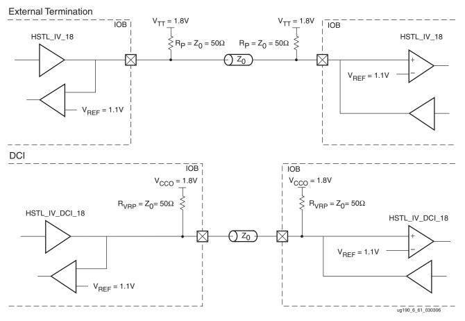
Figure 6-64: HSTL Class IV (1.8V) with Bidirectional Termination
