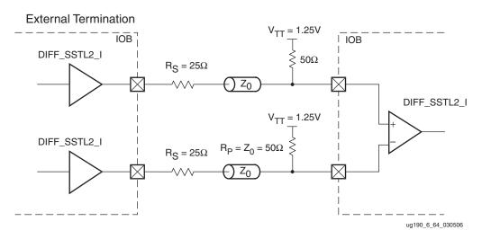
Figure 6-68: Differential SSTL2 Class I Unidirectional Termination
