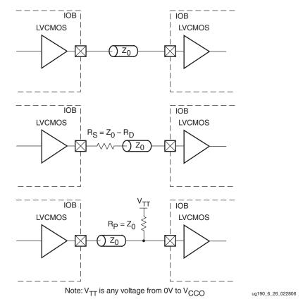
Figure 6-29: LVCMOS Unidirectional Termination
