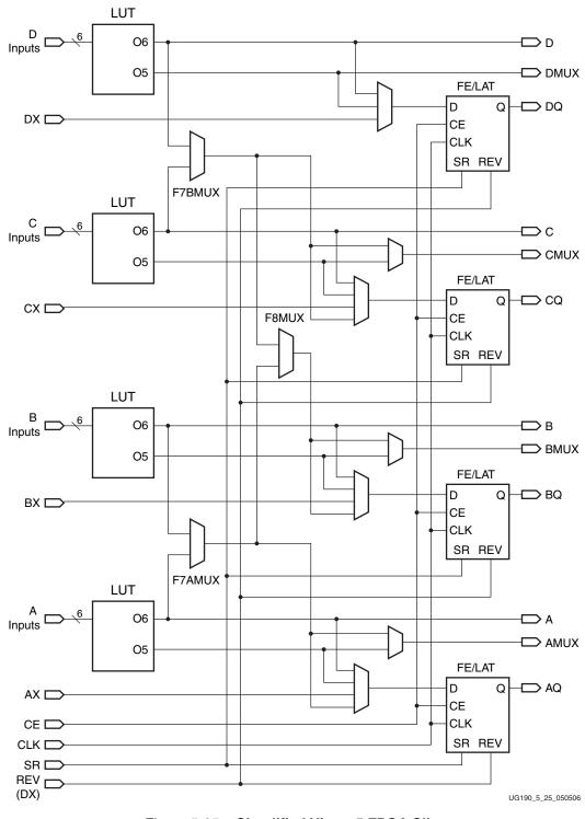
Figure 5-25: Simplified Virtex-5 FPGA Slice
