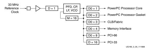
Figure 3-5: PLL as a Frequency Synthesizer
