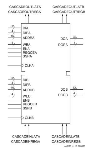
Figure 4-9: Block RAM Port Signals (RAMB36)
