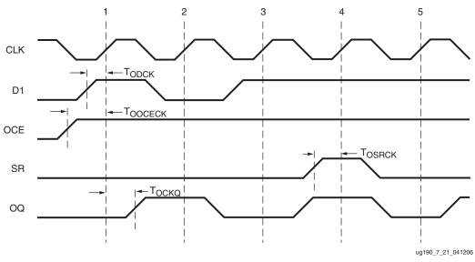
Figure 7-26: OLOGIC Output Register Timing Characteristics
