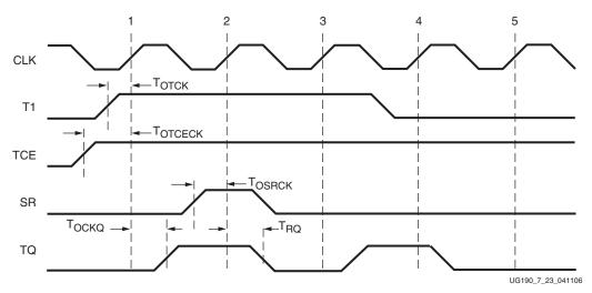
Figure 7-28: OLOGIC 3-State Register Timing Characteristics
