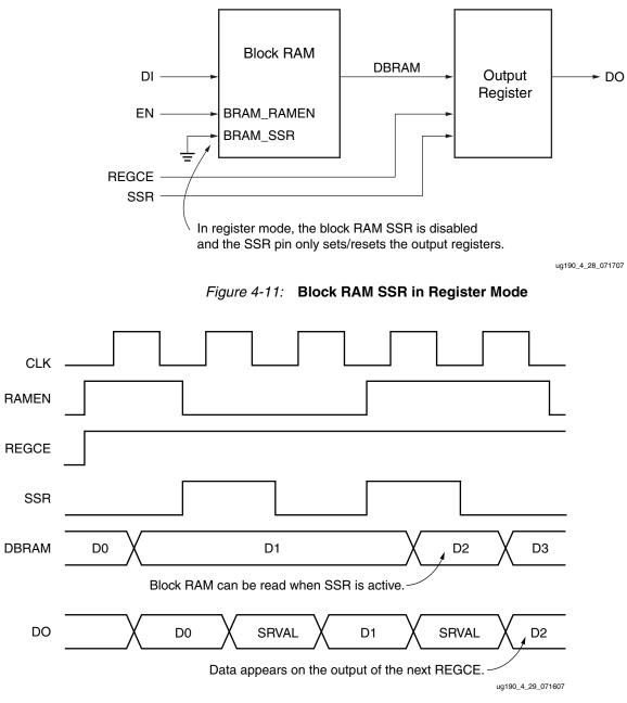
Figure 4-12: SSR Operation in Register Mode with REGCE High
