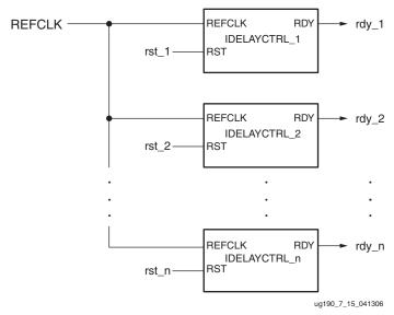
Figure 7-20: Instantiate IDELAYCTRL with LOC Constraint
