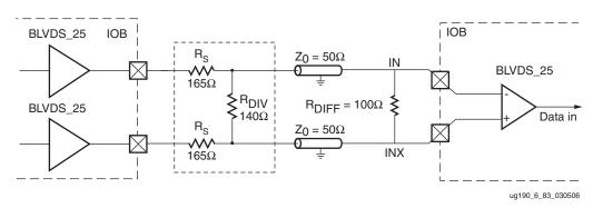
Figure 6-89: BLVDS Transmitter Termination
