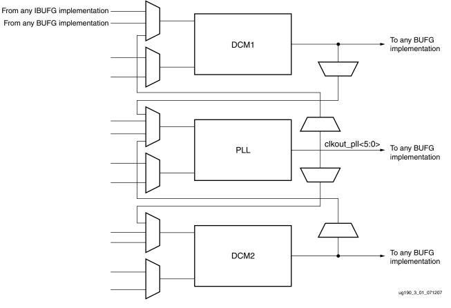
Figure 3-1: Block Diagram of the Virtex-5 FPGA CMT
