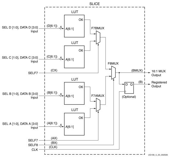
Figure 5-23: 16:1 Multiplexer in a Slice
