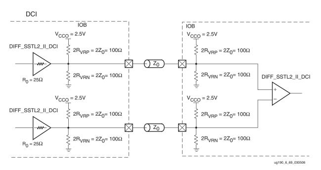
Figure 6-73 shows a sample circuit illustrating a valid termination technique for differential SSTL2 Class II (2.5V) with unidirectional DCI termination.
