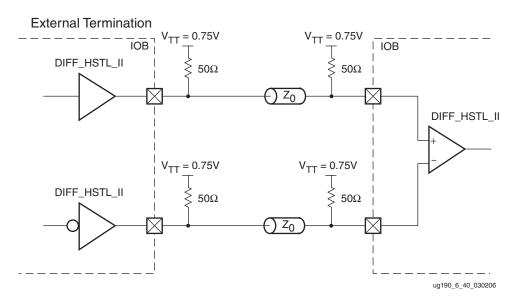
*Figure 6-45:* Differential HSTL (1.5V) Class II Unidirectional Termination
