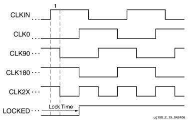
Figure 2-18: Phase Shift Example: Fixed
