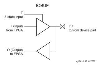
Figure 6-21: Input/Output Buffer (IOBUF) Primitive
