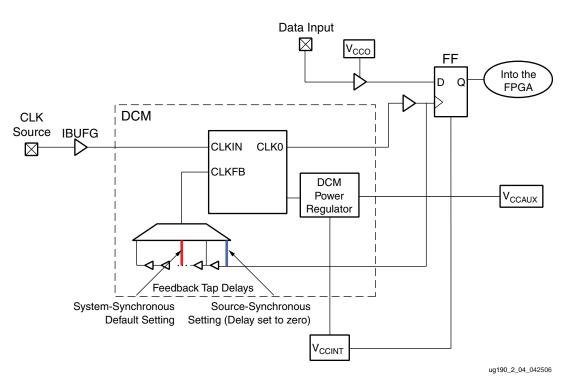
Figure 2-4: DCM and Feedback Tap-Delay Elements
