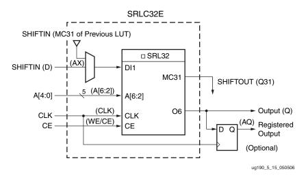
Figure 5-15: 32-bit Shift Register Configuration
