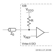
Figure 6-9: Input Termination Using DCI Single Termination
