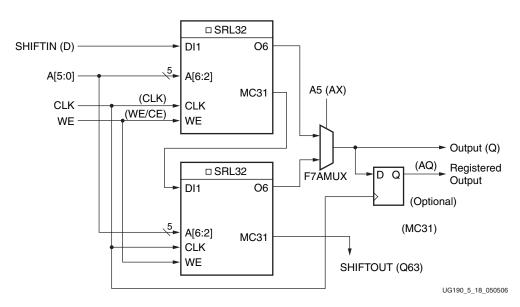
Figure 5-18: 64-bit Shift Register Configuration
