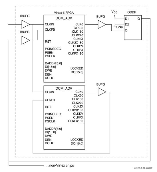
The example in Figure 2-12 shows an interface from Virtex-5 FPGAs to components other than Virtex FPGAs.
