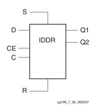
Figure 7-5: IDDR Primitive Block Diagram
