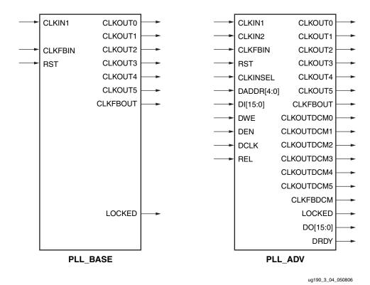
The two Virtex-5 FPGA PLL primitives, PLL\_BASE and PLL\_ADV, are shown in Figure 3-4.
