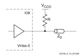
Figure 6-12: Driver with Termination to V<sub>CCO</sub> without DCI
