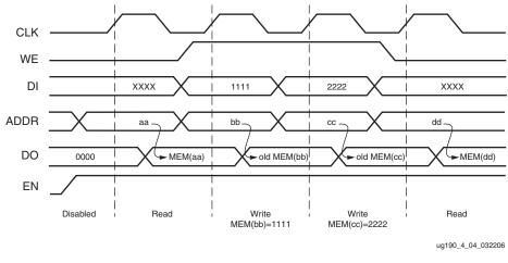
Figure 4-3: READ\_FIRST Mode Waveforms
