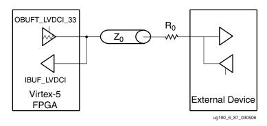
Figure 6-93: 3.3V I/O Configuration
