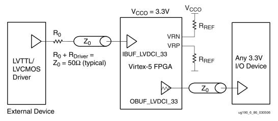
Figure 6-92: Connecting LVTTL or LVCMOS Using the LVDCI\_33 Standard
