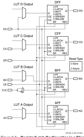
Figure 5-5: Register/Latch Configuration in a Slice
