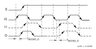
Figure 1-12: BUFGMUX\_VIRTEX4 Timing Diagram
