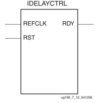
Figure 7-15: IDELAYCTRL Primitive
