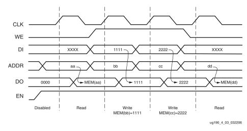
Figure 4-2: WRITE\_FIRST Mode Waveforms
