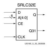
Figure 5-33: 32-bit Shift Register
