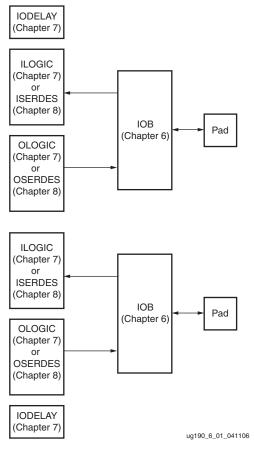
Figure 6-1: Virtex-5 FPGA I/O Tile
