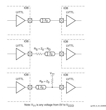
Figure 6-27: LVTTL Unidirectional Termination
