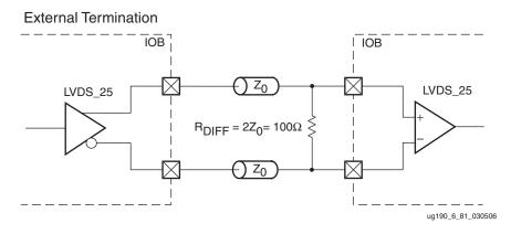
Figure 6-87: LVDS\_25 Receiver Termination
