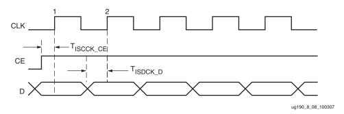
Figure 8-8: ISERDES Input Data Timing Diagram
