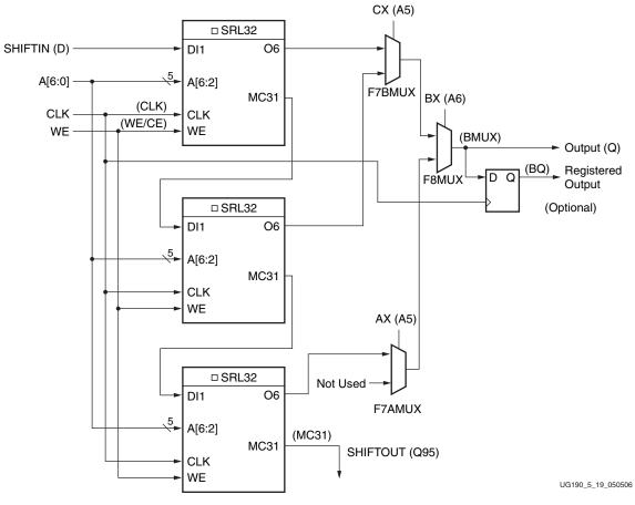
Figure 5-19: 96-bit Shift Register Configuration
