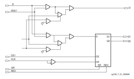
Figure 7-1: ILOGIC Block Diagram
