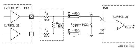
Figure 6-90: LVPECL Transmitter Termination
