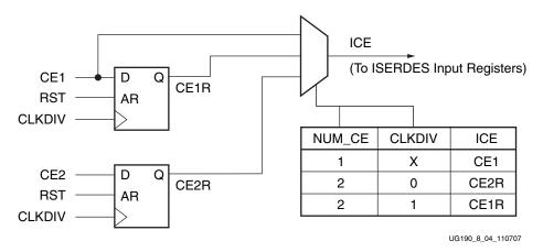
Figure 8-4: Input Clock Enable Module
