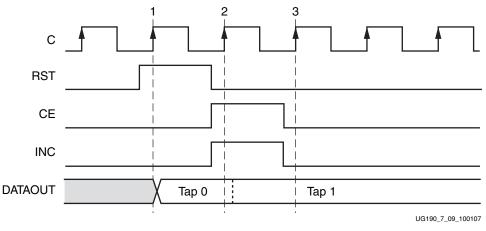
Figure 7-9: IDELAY Timing Diagram
