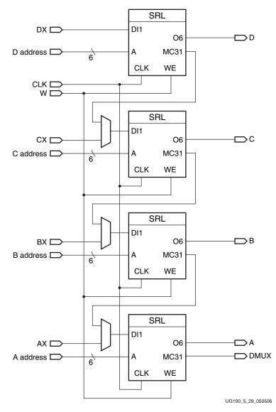
Figure 5-29: Simplified Virtex-5 FPGA Slice SRL
