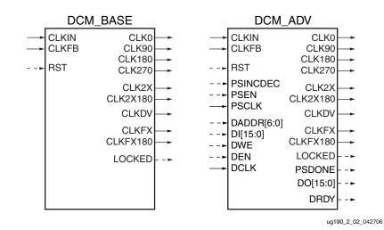
The DCM primitives DCM\_BASE and DCM\_ADV are shown in Figure 2-2.
