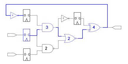
Longest path: FF-AND-NOR-XOR-INV-FF Delay = 3 + 0.25(2) + 2 + 0.25(1) + 4 + 0.25(2) + 1 + 0.25(1) = 11.5 inv delays A path is defined and any series of combinational gates from any flip-flop output to any flip-flop input. This is not necessarily the delay around a loop. A path CANNOT GO THROUGH TWO FLIP-FLOPS.
