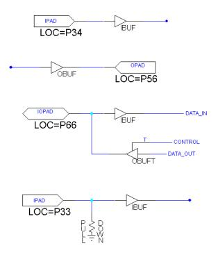
Notice that the OBUFT is a tri-state buffer. Be aware that the control signal "T" is active low, so the output buffer will be enabled (i.e. signals will be output to the pad) when T = 0. When the IOPAD is not being used to output signals, the OBUFT should be turned off (to Z state).
