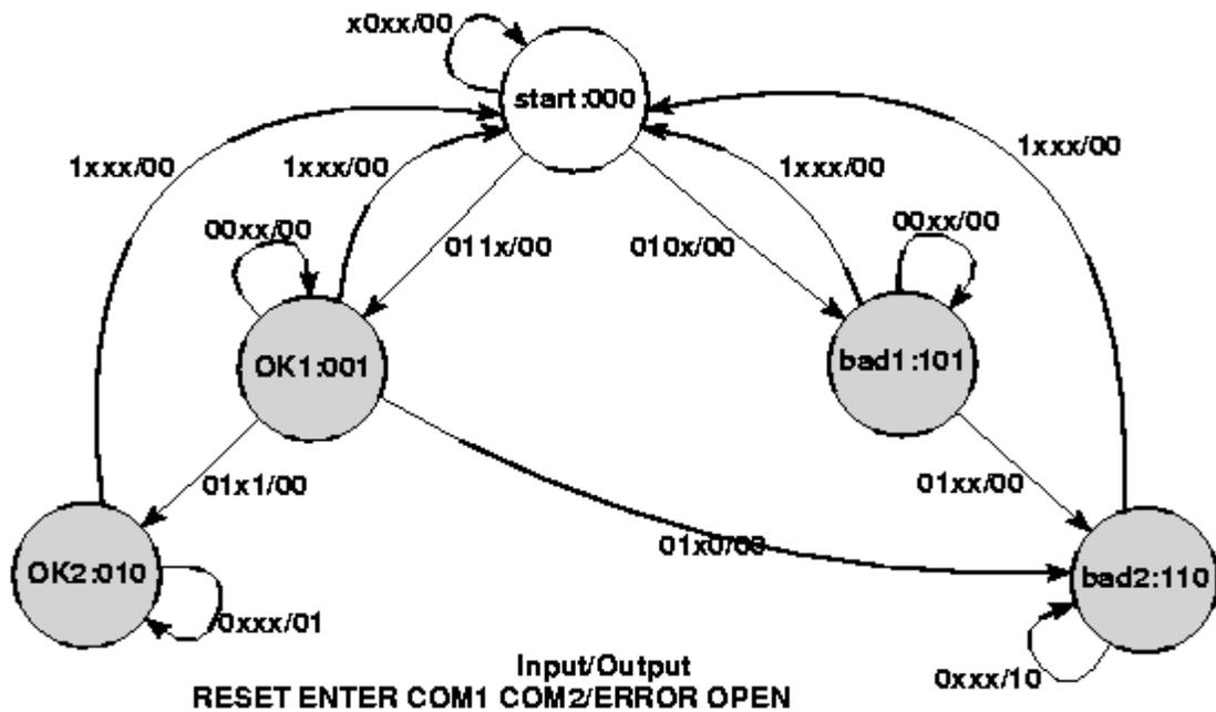
Figure 2: State Transition Diagram
