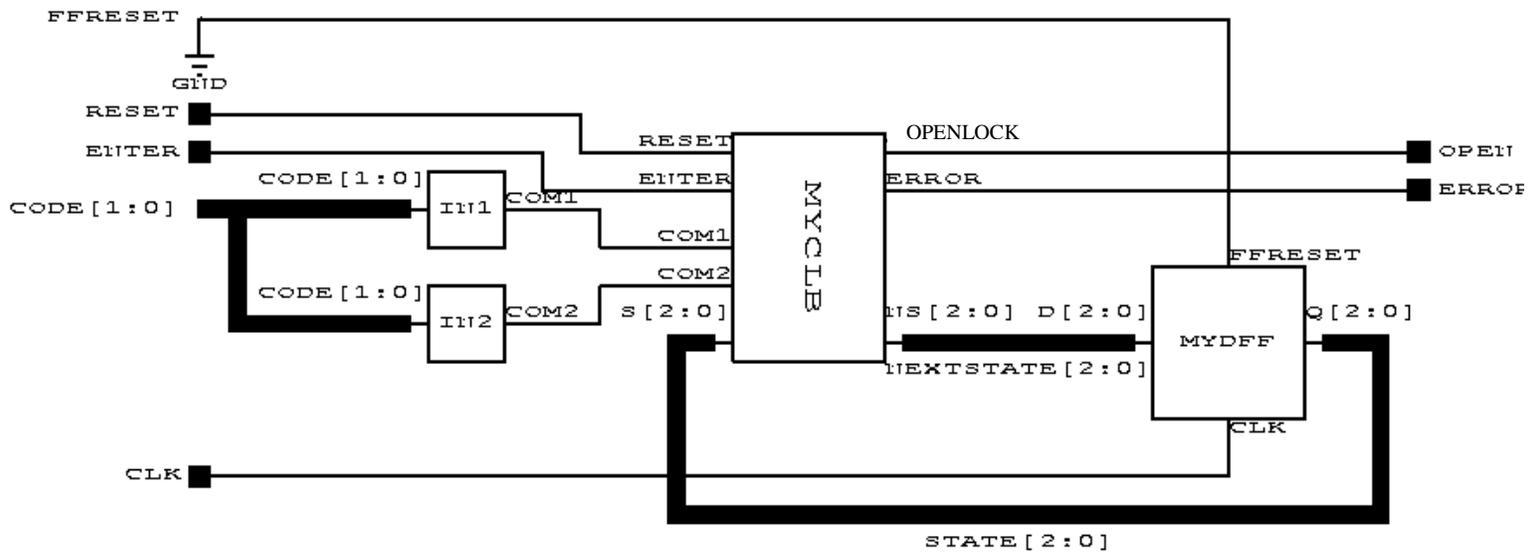
Figure 1: Controller for the combination Lock
