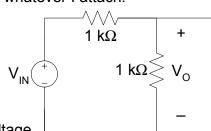
This circuit clearly does not supply the same voltage to any attached load.
