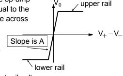
the output is equal to that rail voltage.
