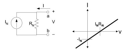
It can model any circuit except a pure independent voltage source, through choice of  $I_N$  and  $R_N$ .
