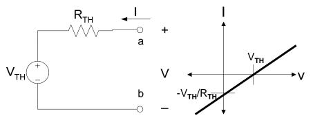
It can model any circuit except a pure independent current source, through choice of  $V_{\rm T}$  and  $R_{\rm T}.$
