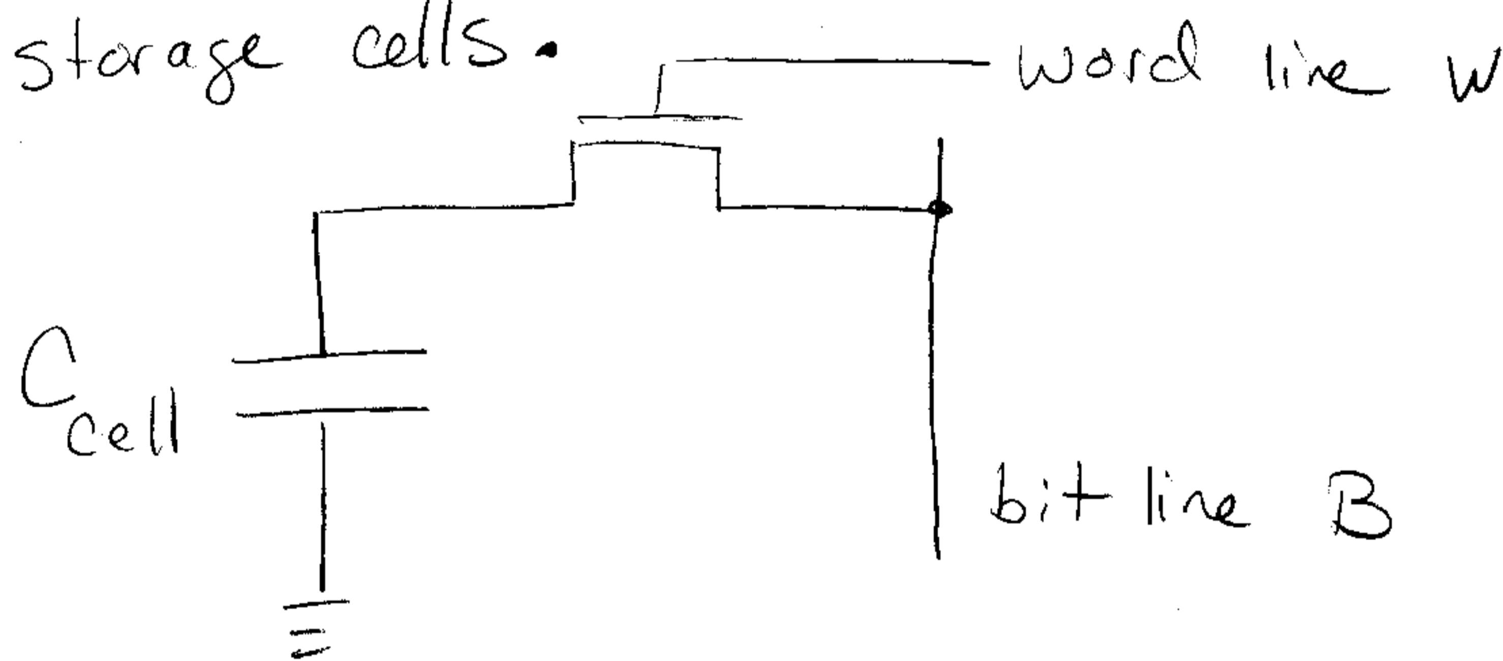
When  $W$  is high, we can write to the cell by holding  $B$  high or low. Capacitor will charge or discharge.
