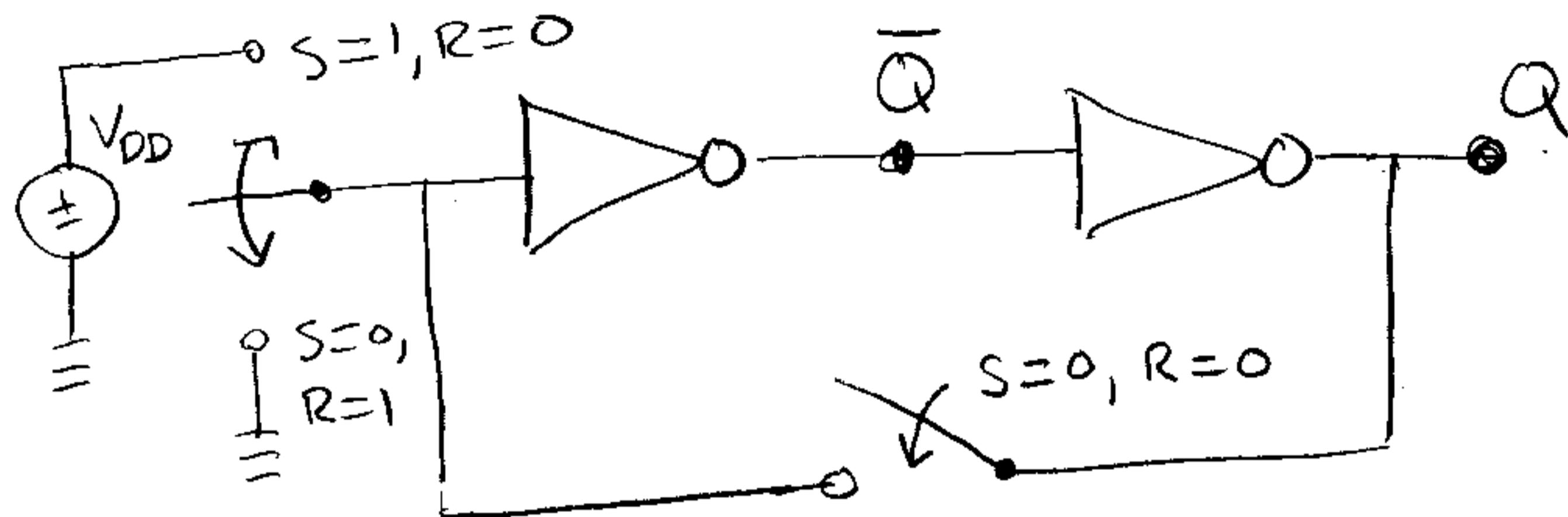
Switches move simultaneously at clock ticks.
