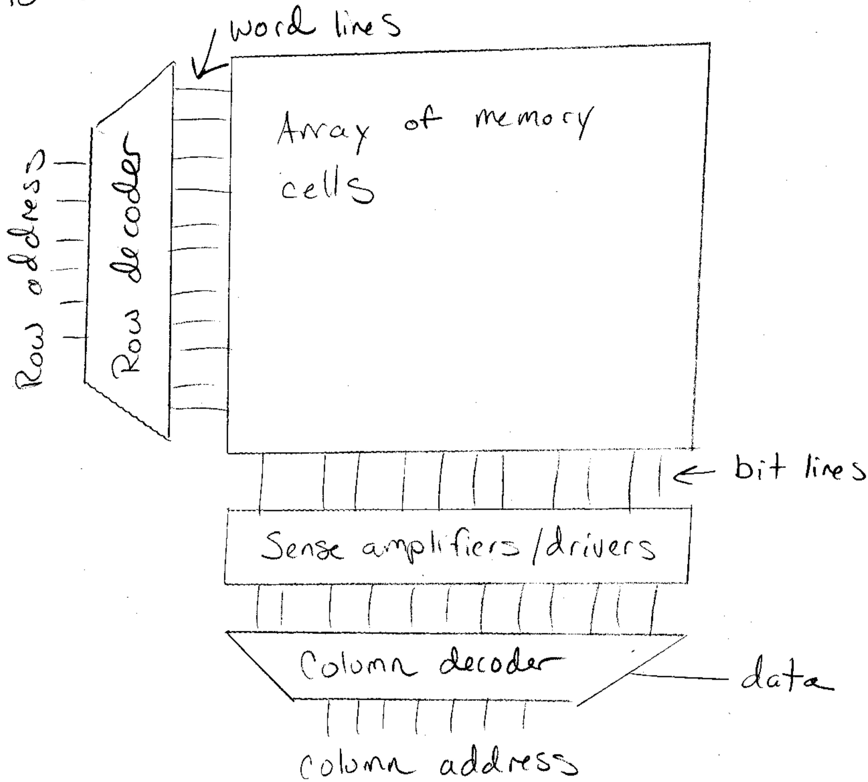
To write a bit, the column and row addresses are specified. The word line for that row is raised to connect the cell. The column decoder activates the driver on the correct bit line.  $B$  is set to 1 or 0, and write occurs as with the flip-flop.
