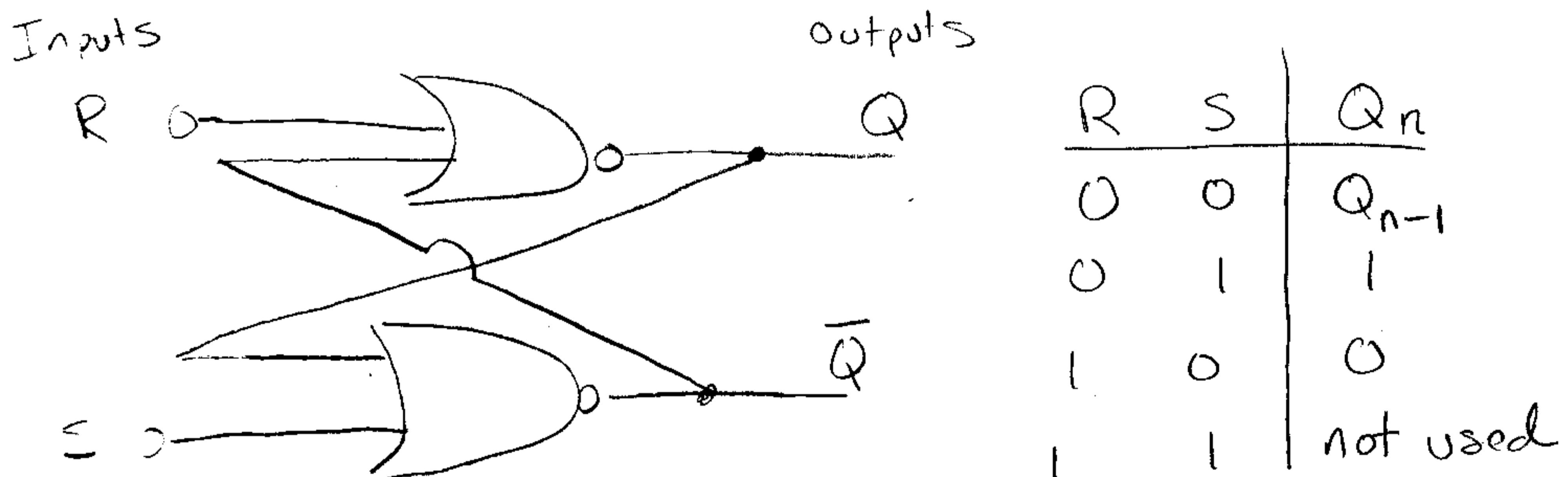
This circuit uses feedback. The output is fed back  $\rightarrow$  the NOR input. So the output at any step  $n$  depends on the output at step  $n-1$  as well as the inputs  $R$  and  $S$ . Steps are controlled by a clock, to be shown.
