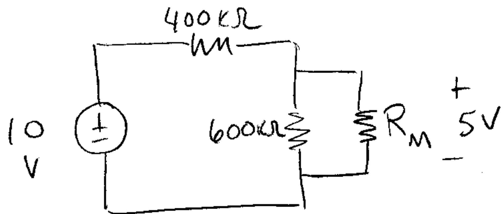
With the voltmeter in, all voltages and currents get changed. Now, the voltage across the  $600\text{k}\Omega$  is 5V.
