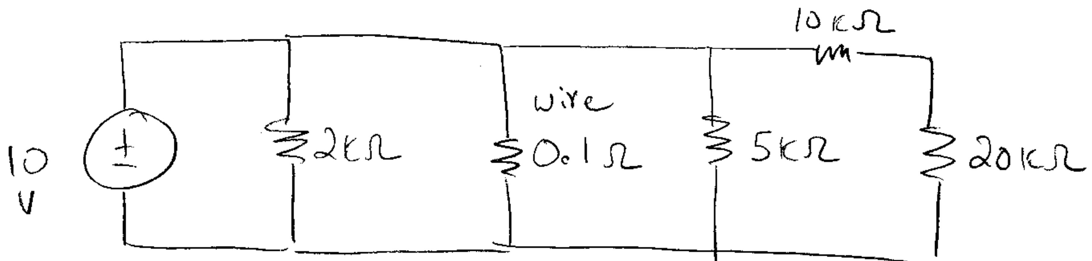
According to Ohm's law, the wire should get 100 A. This wouldn't likely happen — either the wire would melt, the 10 V source would blow a fuse, or the 10 V source would reduce its voltage so that its max current is not exceeded.
