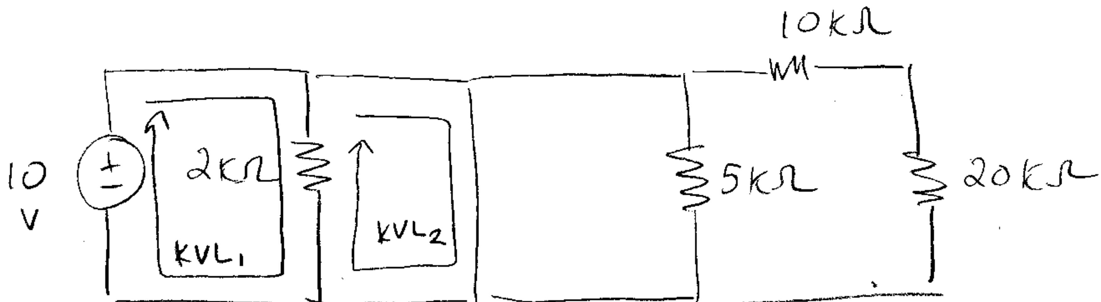
KVL<sub>1</sub> says the 2kΩ resistor should carry 10V.
