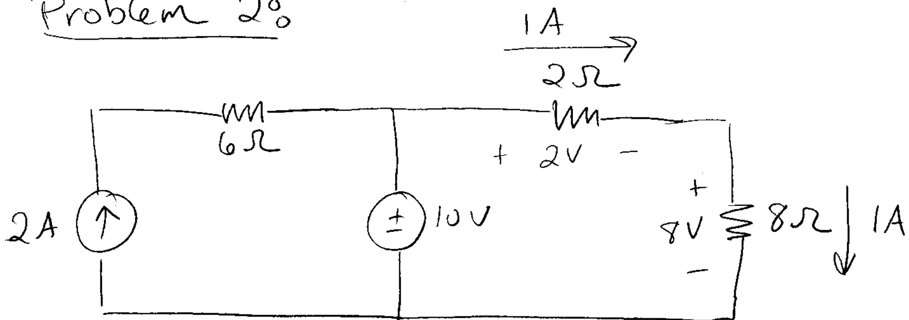
I have 10 V over a pair of series resistors ( $2\Omega + 8\Omega$ ). Using Voltage division, the voltage over the  $2\Omega$  resistor is  $10V \cdot \frac{2\Omega}{2\Omega+8\Omega} = 2V$ . The  $8\Omega$  resistor takes 8 V. The polarity is determined by the 10 V source, so the resistor voltage drops cancel the 10 V source. Using Ohm's law, the current through each resistor is 1A, from + to -. (You could also determine this by combining the series resistors.)
