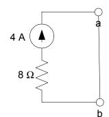
The current flowing from a to b when the terminals are shorted is 4 A, so
