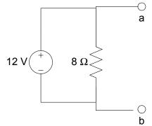
When the terminals are left open, the voltage drop from a to b is 12 V (the source is directly attached from a to b).
