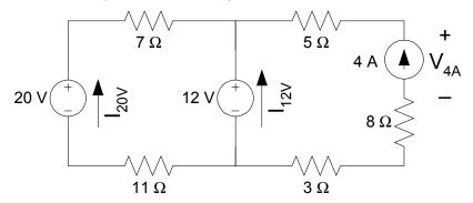
Notice that the the 5  $\Omega$ , 3  $\Omega$ , and 8  $\Omega$  resistors, and the current source, all share the same current. There is nowhere else for the current to go in that path.
