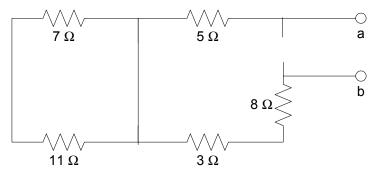
The 7  $\Omega$  and 11  $\Omega$  resistor are in series. They can be combined into a 7  $\Omega$  + 11  $\Omega$  = 18  $\Omega$  resistor.
