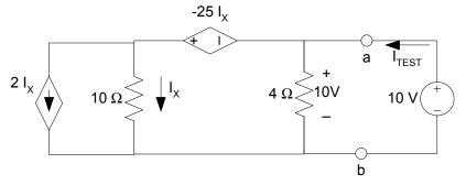
By KVL on the right-hand loop, we see that the 4  $\Omega$  resistor has 10 V as shown.
