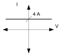
The I-V graph for this circuit is a horizontal line. There is no x-intercept, so  $V_{\text{TH}}$ , and the Thevenin equivalent circuit, do not exist for this example.
