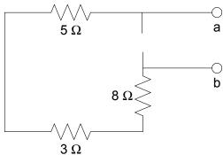
Now, the 5  $\Omega$ , 3  $\Omega$ , and 8  $\Omega$  resistors are in series since they have the same current: no current can go through the hole where the current source used to be. They combine into a 5  $\Omega$  + 3  $\Omega$  + 8  $\Omega$  = 16  $\Omega$  resistor.
