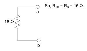
To find  $V_{TH}$ , we find the voltage drop from a to b with the terminals left open.
