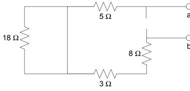
Now, the 18 W resistor is in parallel with a wire. The resistor must have 0 V, or KVL would be violated. So we can ignore this resistor, since it has 0 V and therefore 0 A.
