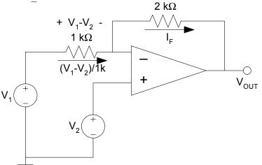
By KCL,  $I_F - (V_1 - V_2)/1k = 0$ , since the current into the op-amp input is 0 A.
