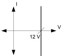
The I-V graph for this circuit is a vertical line. There is no y-intercept, so  $I_N$ , and the Norton equivalent circuit, do not exist for this example.
