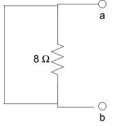
If we find  $R_{TH}$  by replacing the voltage source with a wire, we end up with 8  $\Omega$  in parallel with a wire. Now the resistor must have 0 V and therefore no current, so it can be removed. This leaves only the wire from a to b.
