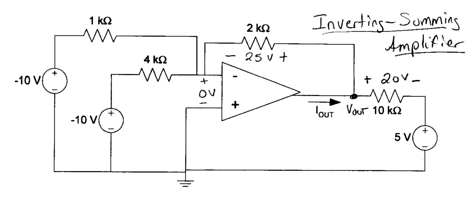
$$V_{OUT} = -\left(\frac{2KSC}{4KSC}\right)(-10 \text{ V}) - \left(\frac{2KSC}{1KSC}\right)(-10 \text{ V}) = 25 \text{ V}$$
