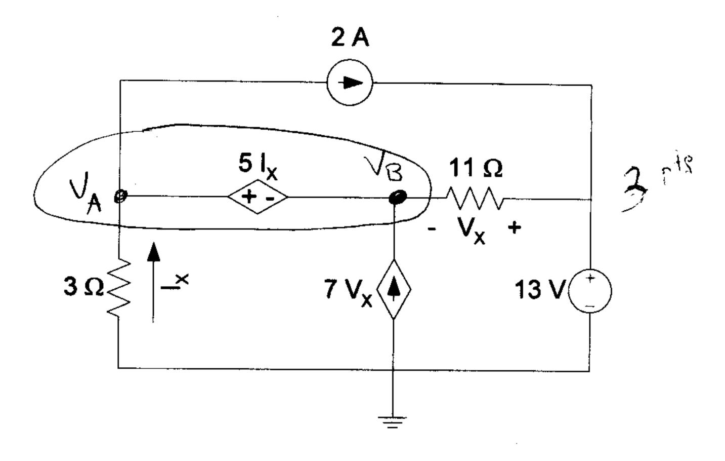
$$\frac{2A - I_{X} - 7V_{X} + \frac{V_{B} - 13}{11} = 0}{V_{A} - V_{B} = 5I_{X}} = 0$$
