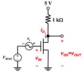
The n-channel MOSFET has dimensions  $W = 20 \ \mu\text{m}$  and  $L = 2 \ \mu\text{m}$ , and  $k_n' = 100 \ \mu\text{A/V}^2$ ,  $V_T = 0.5 \ \text{V}$ , and  $\lambda = 0$ .
