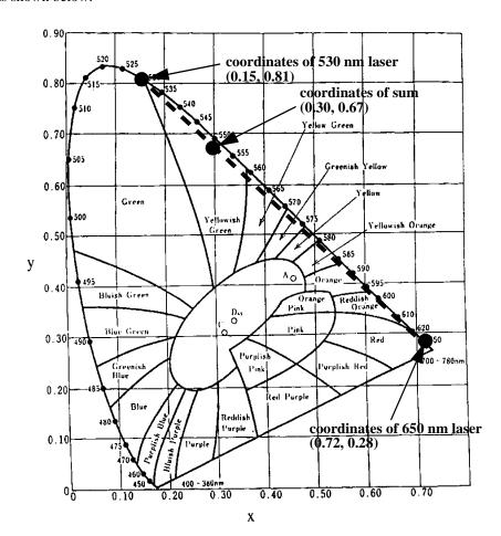
**d**) The X, Y, Z tristimulus coordinates for a light source with spectral radiance  $P(\lambda)$  are given by the following equations;
