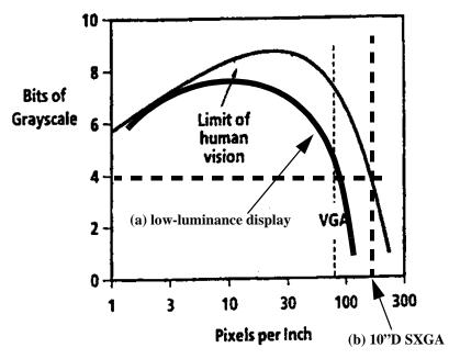
b) For a 10"D SXGA display (1280 x 1024 pixels -- note that the aspect ratio is 5:4, not 4:3!), the number of
