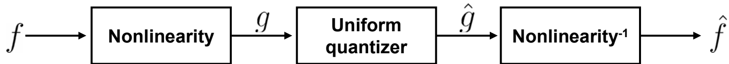
Figure 10.7 Nonuniform quantization by companding.
