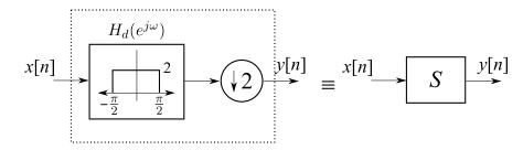
Let  $X_d(e^{j0}) = 1$  and let  $X_d(e^{j\omega})$  be continuous (smooth) at  $\omega = 0$ . What is the output when x[n] is passed through an "infinite number of system S put in serial"? Can you interpret your answer using the noble identities?
