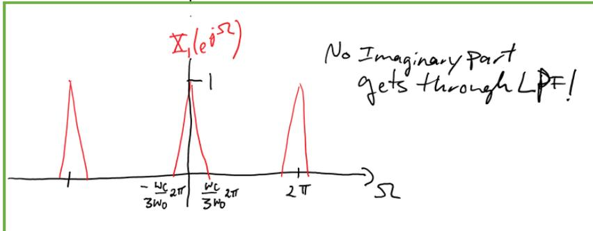
$$r_s[n] = r[n] \cdot \sin\left(\frac{2\pi}{3}n\right) \xleftrightarrow{\text{DTFT}} \frac{1}{2\pi} R(e^{j\Omega}) \circledast \int_{-\pi}^{\pi} \delta\left(\Omega - \frac{2\pi}{3} - 2\pi l\right) - \delta\left(\Omega + \frac{2\pi}{3} - 2\pi l\right) = R_s(e^{j\Omega})$$
