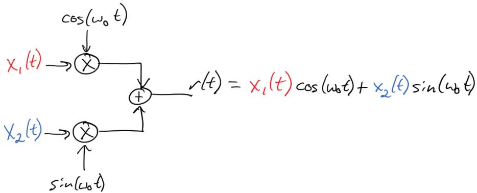
$$R(j\omega) = \frac{1}{2\pi} \underline{X}_1(j\omega) * \pi [\delta(\omega - \omega_0) + \delta(\omega + \omega_0)]$$
