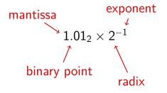
Computer arithmetic that supports this format is called floating point, due to the "floating" nature of the binary point
