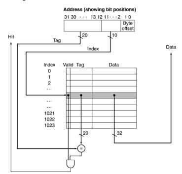
Here is a diagram showing how a directmapped cache determines a cache hit.
